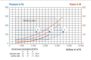
— the limit of the working zone determines the maximum airflow / pressure available at the fan
